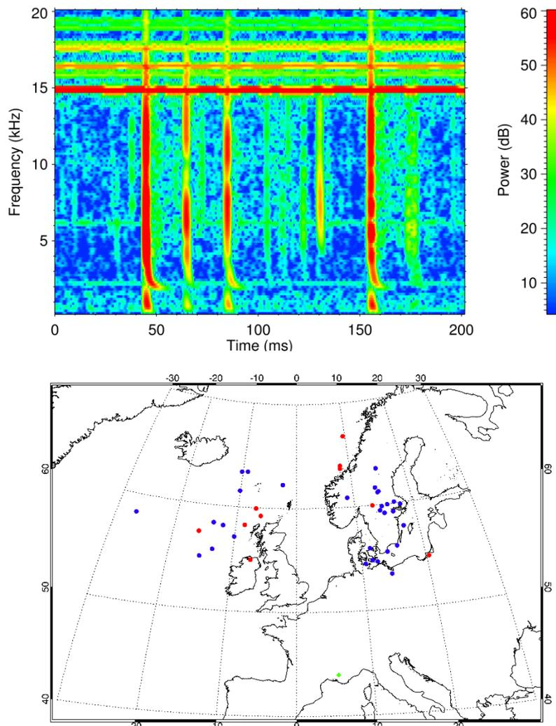
(top) Unusual daytime tweek which is pronounced enough to be suitable for further analysis (9 Jan 2015 at 11:31:41.6; (bottom) Locations of source lightning strokes. Red and blue dots represent positive and negative lightning strokes, respectively; a green cross shows the location of our VLF receiving station.
