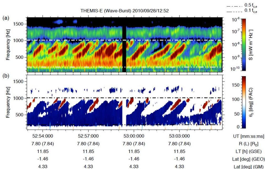
(top) Poynting flux and (bottom) polar angle for chorus emission observed by THEMIS-A on October 29, 2008. The dashed-dotted line marks half of the local electron cyclotron frequency. Orbital coordinates of the spacecraft are given at the bottom.
